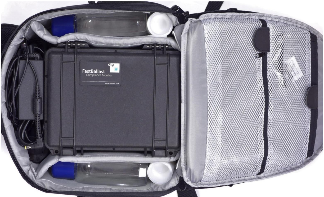
Inner compartment of the backpack (Pasteur pipettes and 30 mL syringes not shown)
